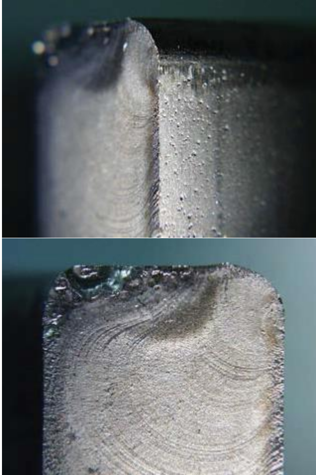
FIGURE 10 - Piston failure by corrosion
