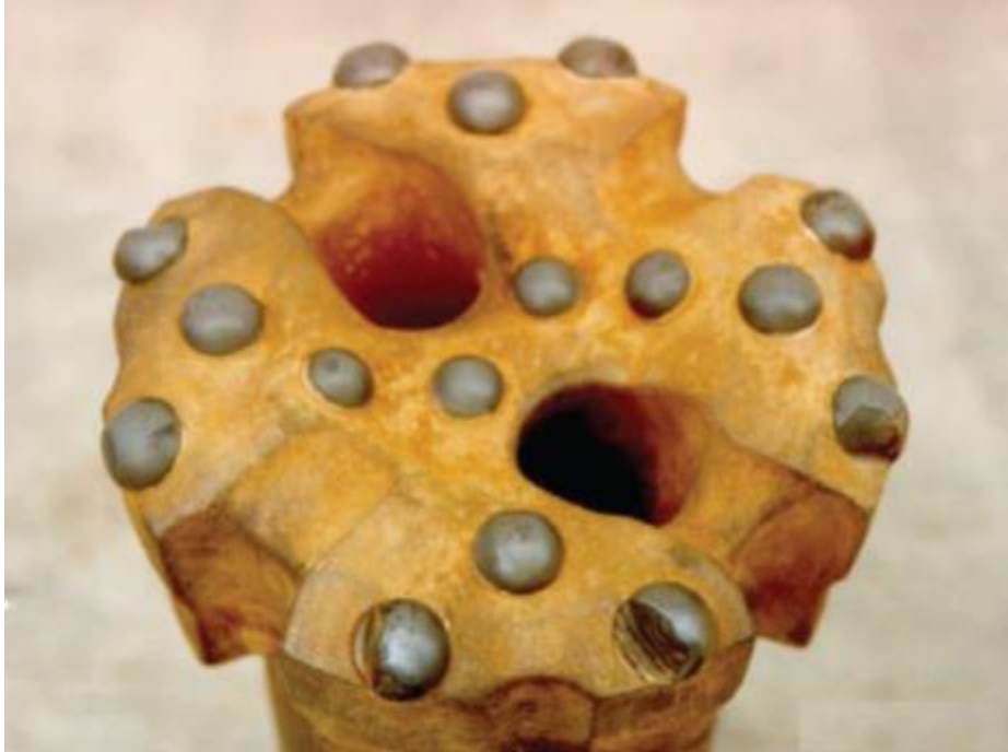
FIGURE 17 - Example of button with “Cusp” failure
