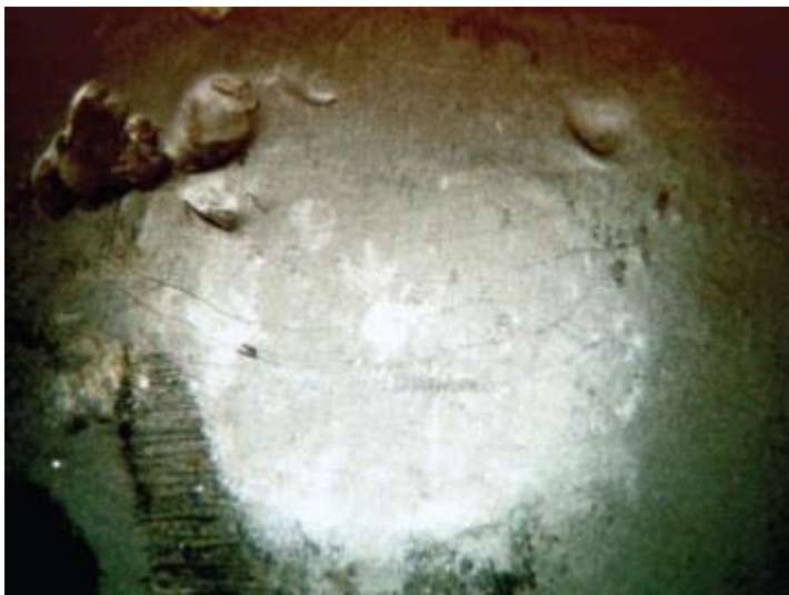
FIGURE 20 - Thermal cracking on tungsten carbide button surface
