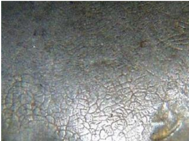
FIGURE 19 - Snake skin on tungsten carbide button surface
