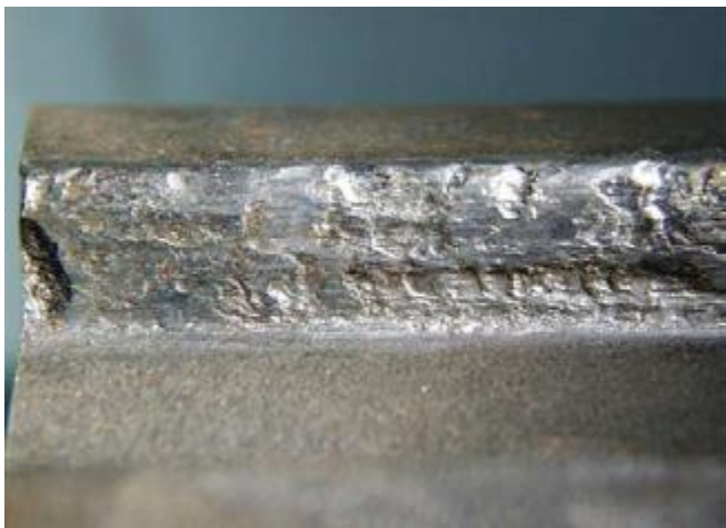
FIGURE 6 - Bit failure due to spline galling
