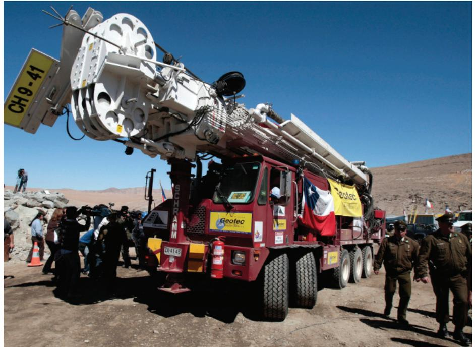
*The Schramm T130XD deep-drilling rig was instrumental in the Chilean mine rescue in 2010, drilling a 28-inch-wide hole through solid andesite rock to extract 33 miners.*
