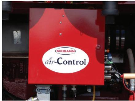
*Schramm's air-CONTROL system manages a vehicle's compressor and variable speed fan to maintain constant pressure and temperature.*
