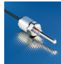
*ifm temperature sensors are Pt1000 RTD based units that are ideal for monitoring hydraulic fluid. They feature a high accuracy 0.5V to 4.5 V analog output.*
