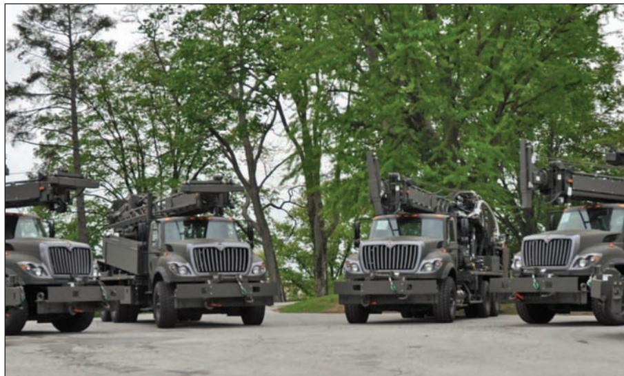
hole hammer drilling methods. The truck engine provides power for all the hydraulic, mud, and air systems.
