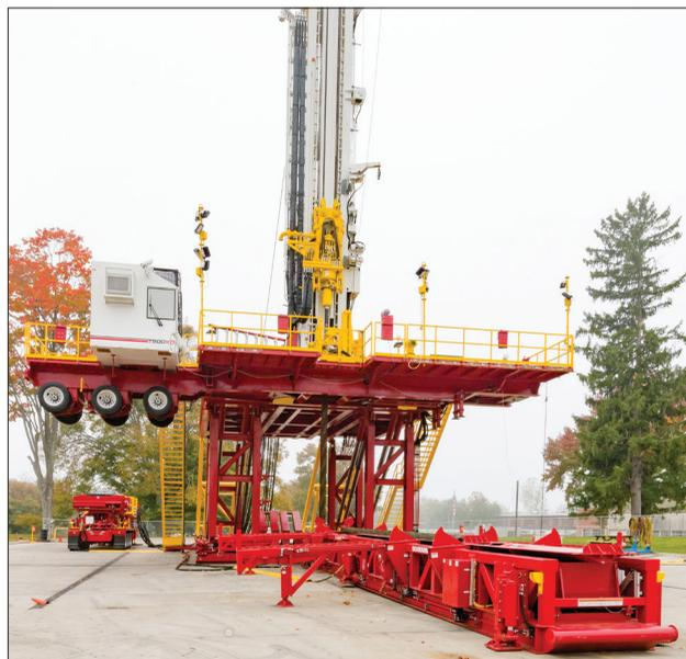
**With a 500,000-lb hook load and world-class technology, the T500XD is the right tool for both horizontal and directional drilling. (Source: Schramm)**
